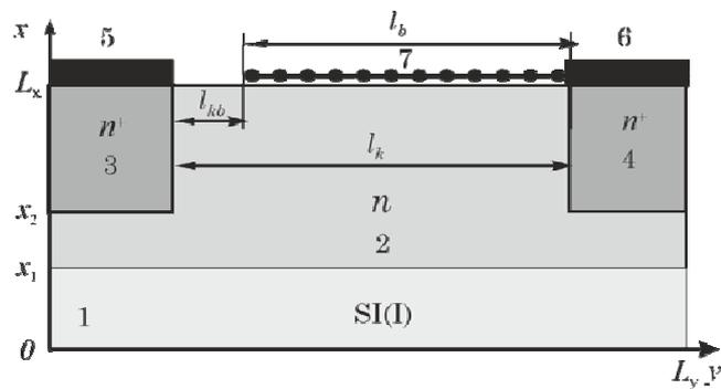
Fig. 1. Diode structure: semi-insulating substrate (1), channel (2), heavily doped contact area (n<sup>+</sup>) (3,4), cathode (5) and anode (6) - metal contacts, MoS<sub>2</sub> monolayer (7).
