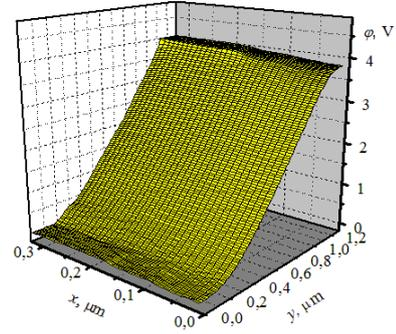
Fig. 2. Distribution of electrostatic potential in a diode,  $N_s = 0$ ,  $l_{bb} = 0.16 \mu\text{m}$ .
