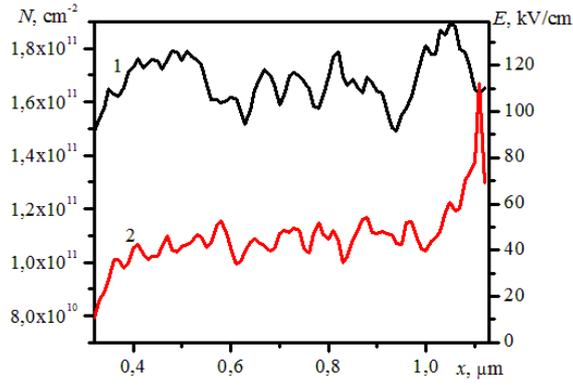
Fig. 4. Static distribution of surface electron concentration (1) and electric field strength ( $E_y$ ) (2) in a monolayer,  $N_s=0$ ,  $l_b=0,16 \mu\text{m}$ ,  $U=0 \text{ V}$ .
