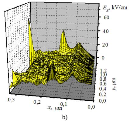
Fig. 3. Distribution of  $E_y$  a) and  $E_x$  b) - components of electric field intensity,  $N_s = 0$ ,  $l_{bb} = 0.16 \mu\text{m}$ .
