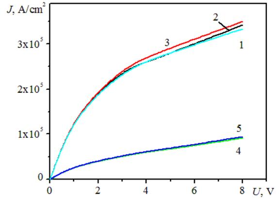
Fig. 6. Dependence of current density on voltage for diodes with 2D- $\text{MoS}_2 - 3\text{D}$  GaN heterojunction, donor concentration  $N_s=10^{11} \text{ cm}^{-2}$ : 1 -  $l_b=0,8 \mu\text{m}$ ; 2,4 -  $l_b=0,64 \mu\text{m}$ ; 3,5 -  $l_b=0,48 \mu\text{m}$ .
