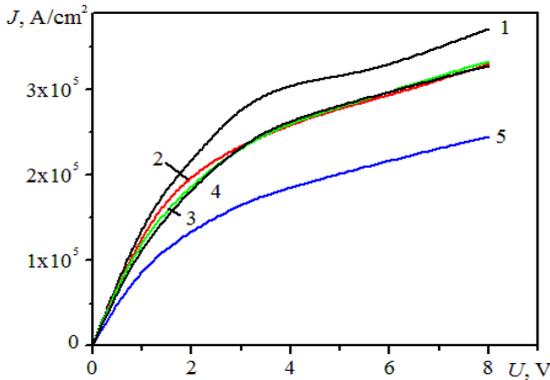
Fig 5. Dependence of current density on voltage for diodes based on GaN without a heterolayer and with a heterolayer with a thickness of  $0,8 \mu\text{m}$  ( $l_b=0,16 \mu\text{m}$ ): 1 – diode without heterojunction; 2-5 diode with 2D- $\text{MoS}_2 - 3\text{D}$  GaN heterojunction: 2-  $N_s=0$ ; 3, 5-  $N_s=10^{11} \text{ cm}^{-2}$ ; 4-  $N_s=10^{12} \text{ cm}^{-2}$ .
