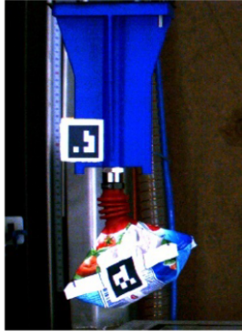
Fig. 14: Swinging packed viscous product in fluid picked by suction cup. Source Blue Print Automation, Woerden, The Netherlands
