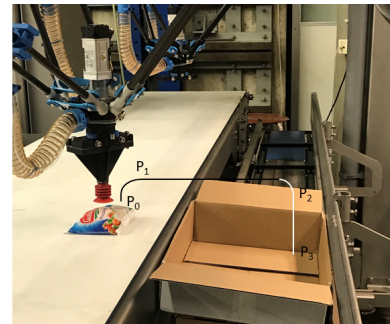
Fig. 13: Delta robot setup and path for pick and placement of food-packaging. Source Blue Print Automation Woerden, The Netherlands.
