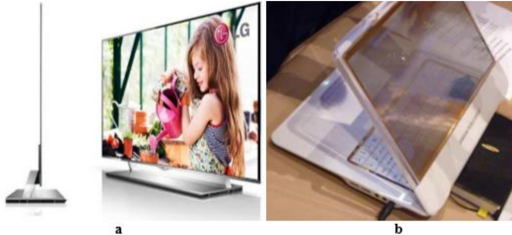
Figure 8: a: Full-HD AMOLED TV (4mm thick and weighs just 3.5 Kg); b: Transparent OLED Laptop
