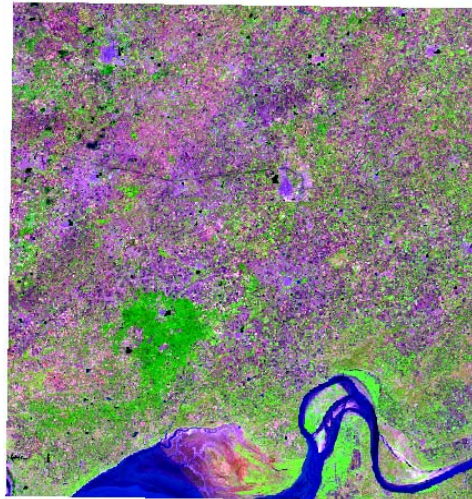
Fig. 3 False Color Composite created from LISS III Band Data
