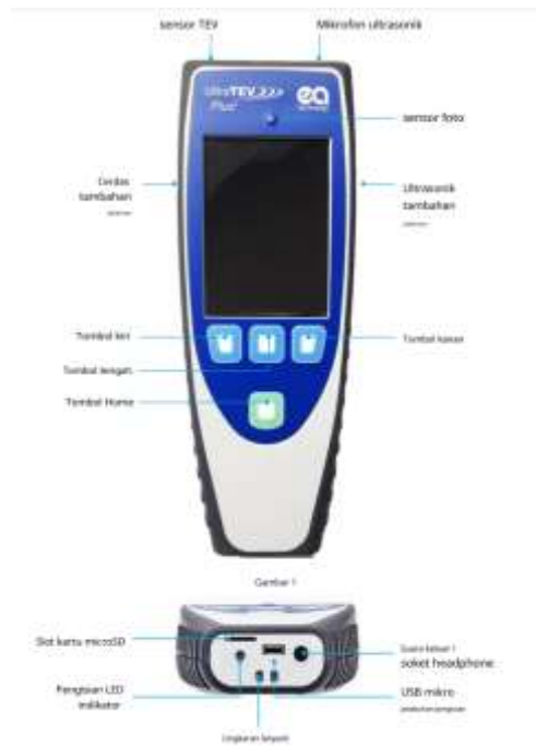
Gambar 3 Peralatan UltraTEV Plus 2
