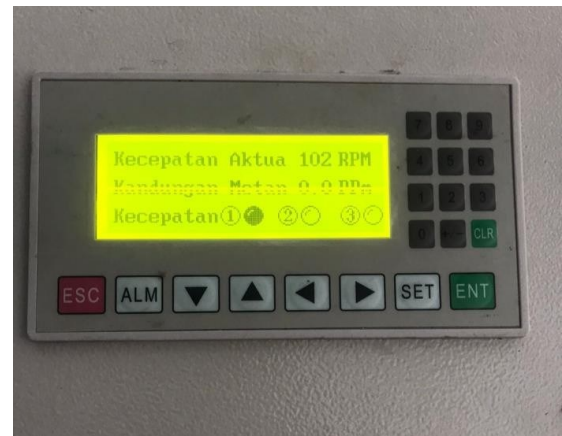
Figure 9 UI display results on HMI OP320
