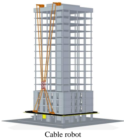
Figure 7. Conceptual view of a cable robot (Orange) working on a building. The platform hosting the MEE is coloured red.
