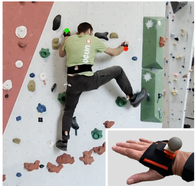
Fig. 1. Experimental evaluation in a bouldering scenario with IMUs and ground truth markers attached to the climbers’ hands, feet and hip. The approach presented in this paper uses the hand IMUs only and estimates the positions of both hands separately. The estimates for the depicted situation are marked with green and red dots.
