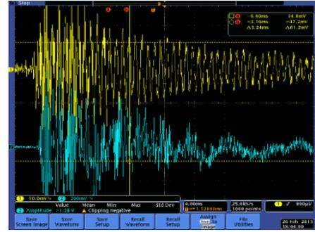
Fig. 2 Disturbance in the transmittance of the LPG gratings due to the passage of the traveling longitudinal pulse.
