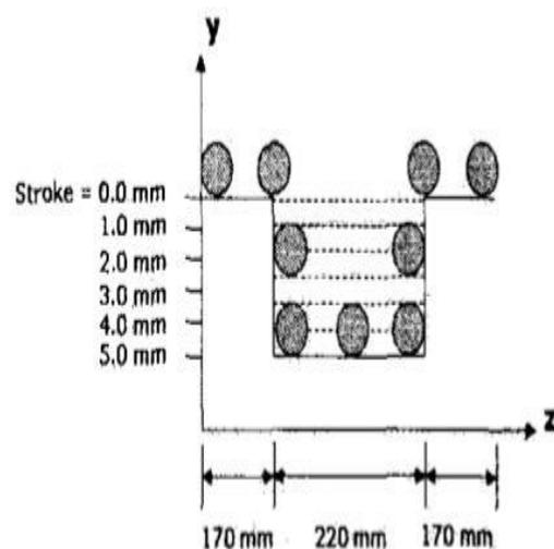
fig.-2 Pulley path in bending experiment
