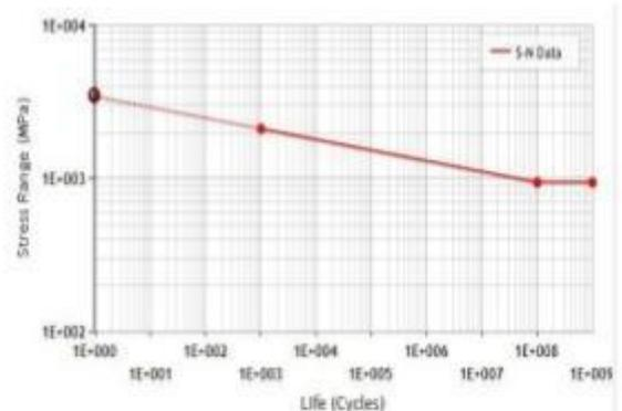
Fig. 6 – S-N Diagram of Structural Steel
