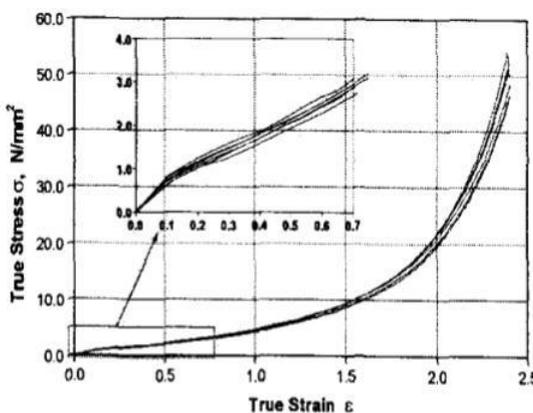
Fig. 5 - Stress & Strain Relation of Polyurethane Rubber used in the Experiment.
