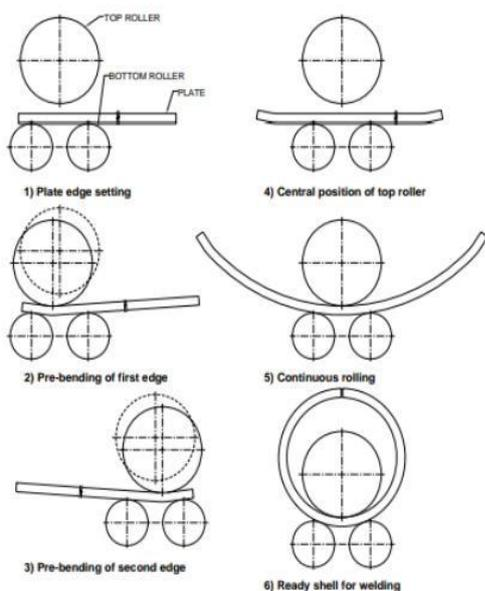
Fig.-1 Pulley sequence for fixed upper pulley gap
