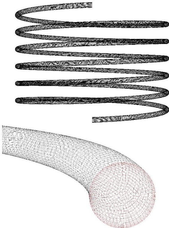
Figure 2. Computational domain and mesh
