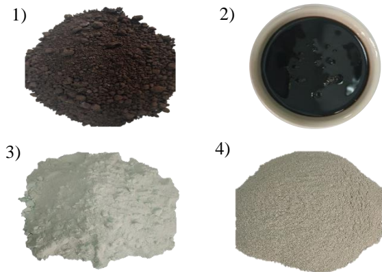
Fig. 1. The initial components for new soil amendments production: 1) leonardite; 2) molasses; 3) \text{FeSO}_4 ; 4) bentonite
