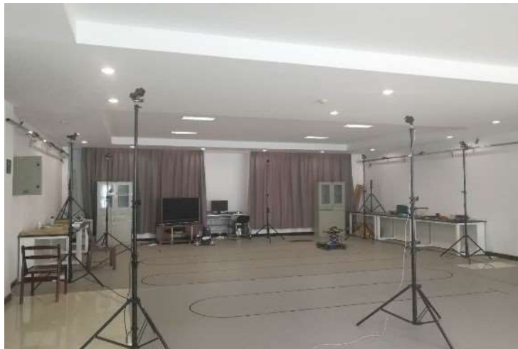
Figure 3 System placement scheme
