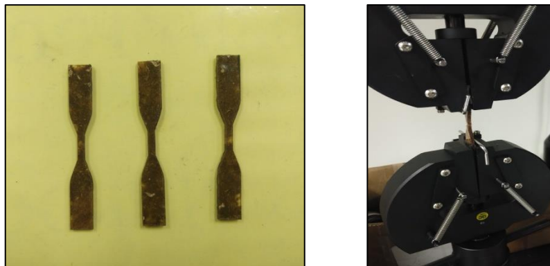
FIGURE 1 Type V Dog Bone Specimen used for Tensile Testing
