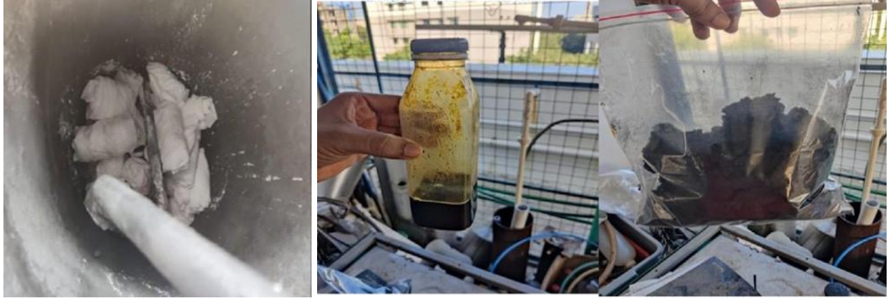
Fig.2. Fresh rolled pads as feed (A), obtained Oil and Pyro-char (B)
