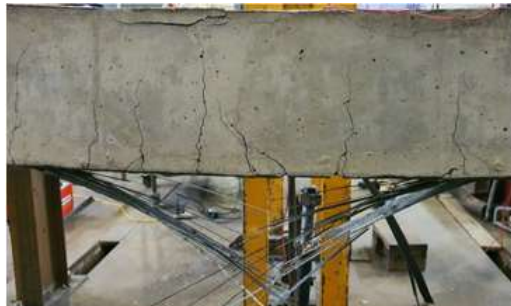
Fig 8. Failure mode of D-1 specimen
