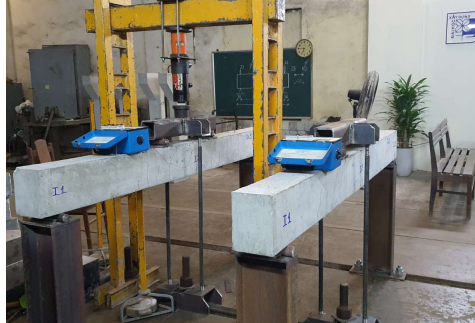
Fig 4. Pre- loading on D-1 beam
