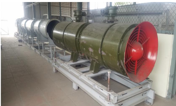
Fig.1. Experimental apparatus for determination of duct resistance
