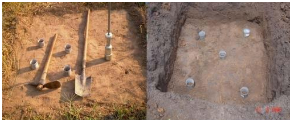
Fig. 15. Uhland sample and field soil sampling, showing the pit
