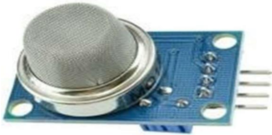
Fig 4.3 MQ3 GAS Sensor.
