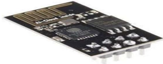
Fig 4.6 Wi-Fi Modem ESP 8266.
