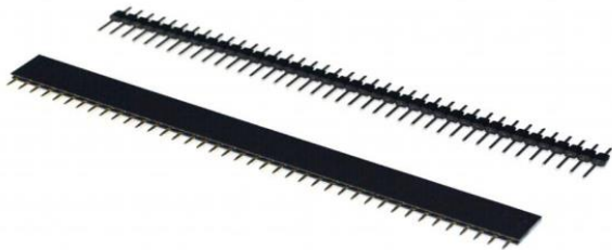
Fig. 5. Male Header, Female Header
