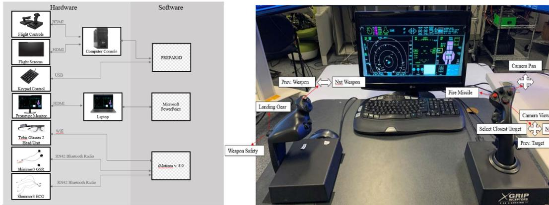
Figure 2: Hardware-software Integration along with display and controls
