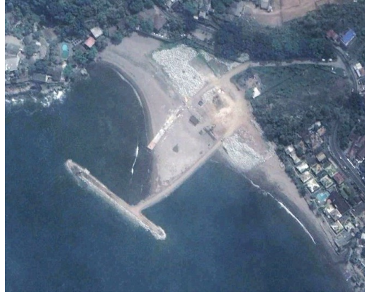
Fig. 6: The accelerated forming of tombolo due to the backfill for material access roads during the construction period (September 2018) that is not modelled in this study.
