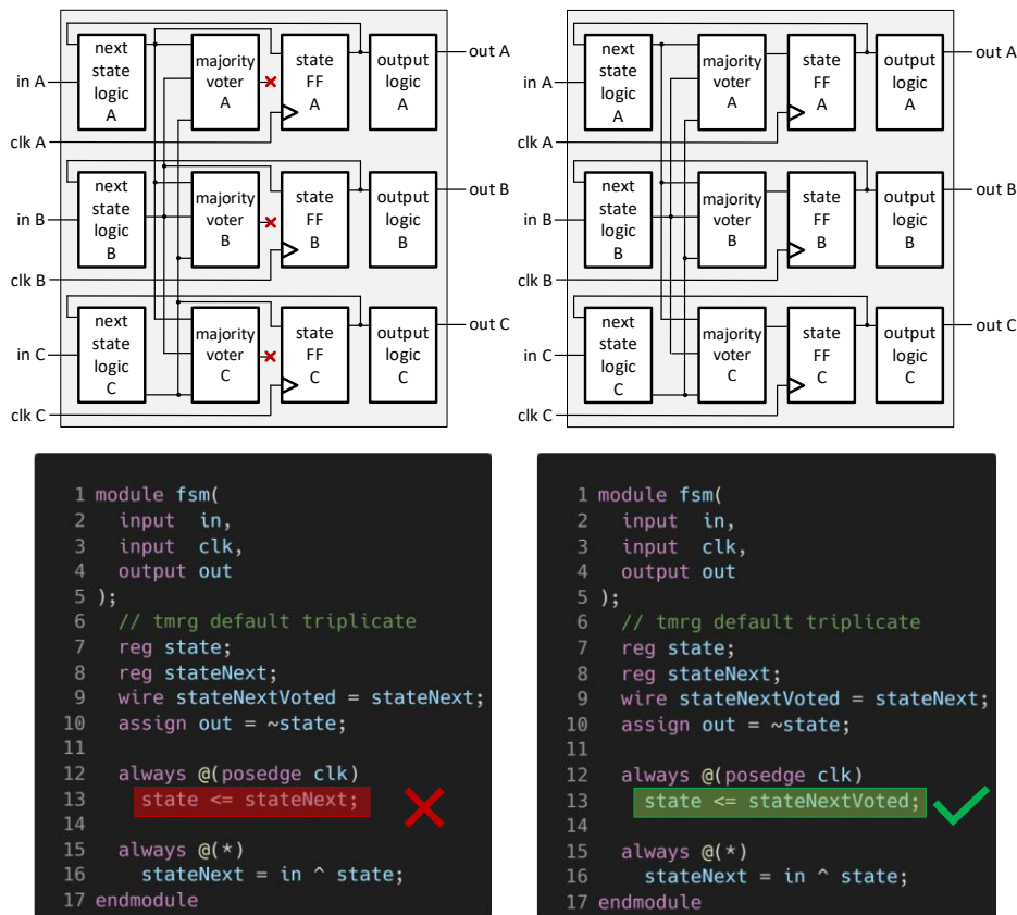
Figure 12 Illustration of a bug caused by the incorrect use of a non-voted signal instead of a voted signal by the designer. The circuit and code on the left display the design with the bug (marked with a red X). The circuit and code on the right show the correctly triplicated design.
