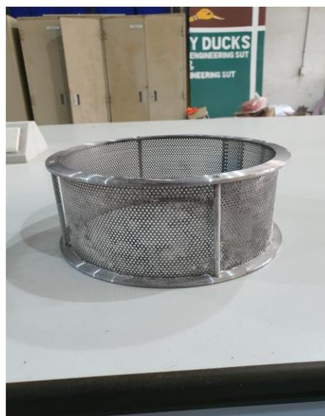
**Figure 1** 1 mm sieve in a rice grinder
