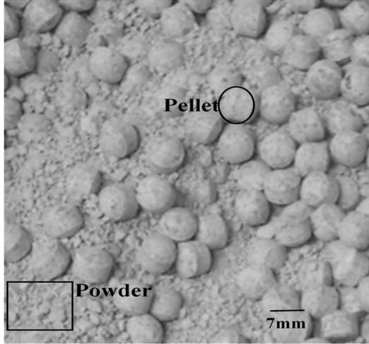
Fig.1. MX-80 bentonite mixture of pellets and powder.
