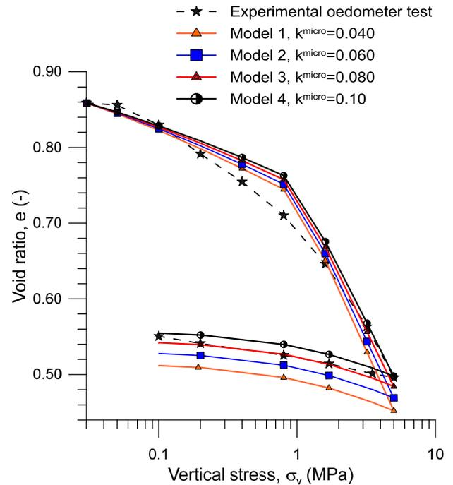
Fig. 7. Evolution of void ratio against axial stress. Experimental and modelling results.
