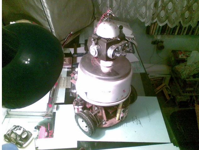
Fig.1. First Iranian pedagogic Robot called “ PARS-1B ”, with AI Graph Search Algorithm to track and find barriers and targets. Developed by Author, in Sharif University of Technology, E.E. Dept, year 1986.
