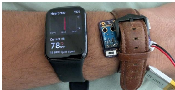
Figure 5. Experimental setup showing the prototype positioned inside a wristwatch strap and worn alongside a Mi Band 9 Pro for preliminary validation of heart-rate and SpO 2 measurements
