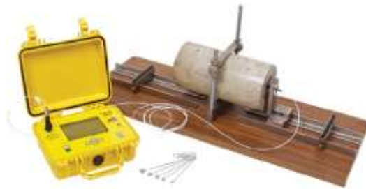
Figure 2. Emodumeter setup for Young's Modulus of Elasticity measurement
