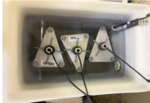
Figure 1. Equipment frame settings for CTE Measurement
