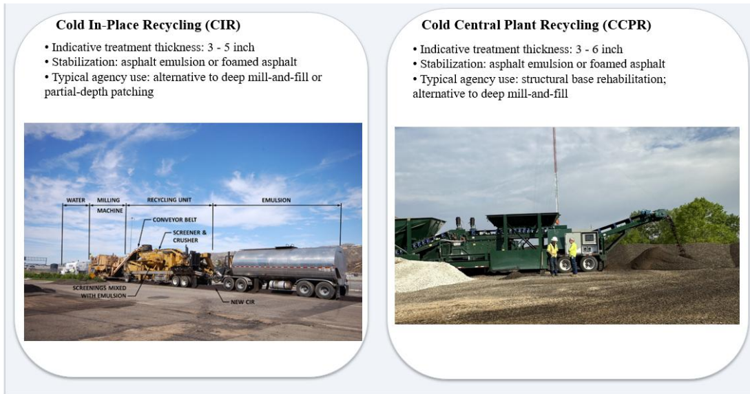
Figure 2. Cold pavement recycling options
